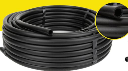
Landscape Products 1/2-inch textured poly swing riser pipe is made from linear low density polyethylene with added elastomers for extra strength. This product is tough and resilient, while flexible at the same time for ease of use. This pipe is used with barbed fittings to attach sprinkler heads to buried laterals. Connect the pipe with fittings to provide a flexible joint that helps prevent damage to the buried pipelines if the sprinkler is hit by maintenance equipment.
